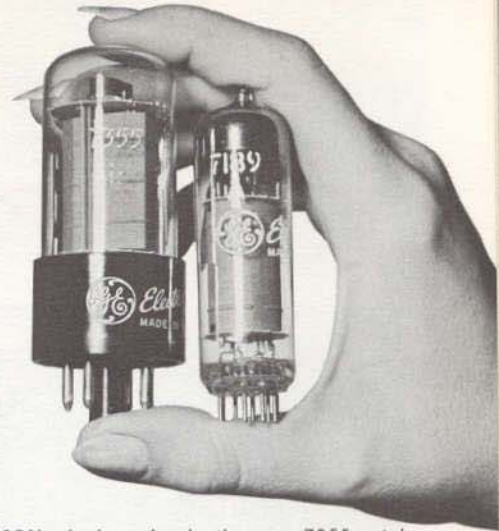
COMPARISON of plate size in the new 7355 octal beam pentode (left), and the 7189A miniature beam pentode (right). The tubes have design maximum plate dissipation ratings of 18 and 13.2 watts, respectively.
